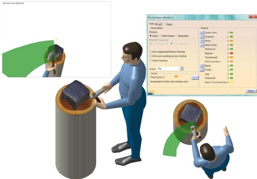
Fig. 9 - Ergonomics Design & Analysis: a-human with hammer, b-vision space, c-results of RULA analysis, d-top view with reach position analysis
